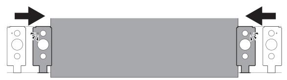
• To print on thin or soft media, swap left and right edge holders and attach them as shown in the figure below so that the hole on the edge holder is located on the inside of the holder. This will hold down wider area on roll media.
