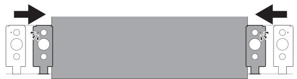
• To print on thin or soft media, swap left and right edge holders and attach them as shown in the figure below so that the hole on the edge holder is located on the inside of the holder.
